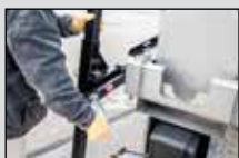
Patent pending lift mechanism with replaceable jack for serviceability and long life
