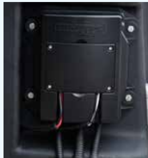
Reduced power loss and corrosion with direct drive and vibrator connections (right image with cover removed to show connections)
