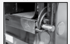
3008560 - Optional Dump Tail Gate Latch Kit
