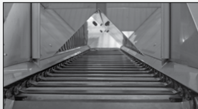
24" wide conveyor chain with 1/4" bars
