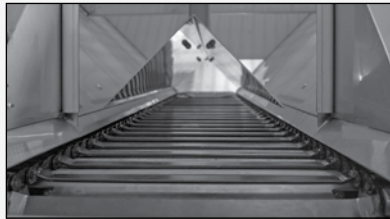
24" wide conveyor chain with 3/8" bars
