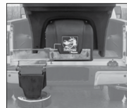
Swing-away chute for bulk unloading
