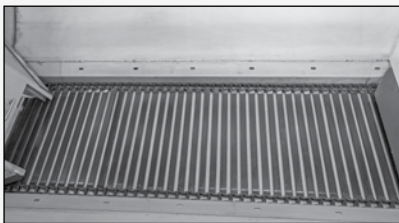
30.25" wide conveyor with 1/2" bars
