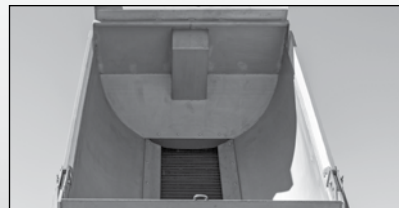
Unique, roll-formed sides and cross memberless floor design
