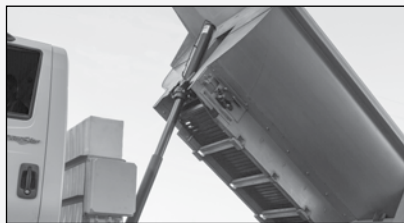
Mailhot® multi-stage, double-acting, nitrided cylinder, trunnion-mounted hoist
