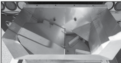
"Hex flow" chute and 24" spinner with adjustable baffles for optimal spread pattern
